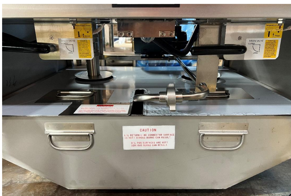
Figure 8: Oil Collection Tank
